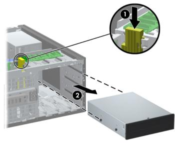
• To remove a 5.25-inch drive in the minitower configuration, pull up on the green drivelock mechanism (1) for that specific drive and slide the drive from the drive bay (2).
